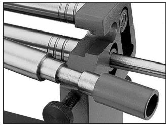
Figure 32. Releasing top roller (T21324 shown).
